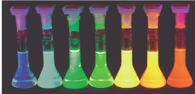
Figure 1.3: Different emission colors from different sizes of CdSe nanoparticles. The nanoparticles were capped with ZnSe. (Adapted from [15]).
